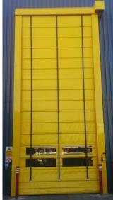
**Opening Activation:** To activate the door opening the following methods can be used individually or in parallel: induction floor loops; photo-electric cells; radar; hand-held or vehicle mounted transmitters; push button (single, double or mushroom) and pull cord. Where pedestrian access is permitted or unavoidable please consult us for advice on stand-off sensing devices or alternative methods of protection.
